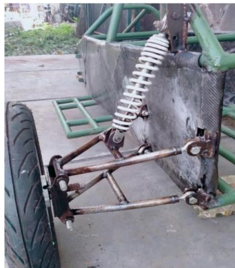
Figure 14. Rear suspension that has been installed on the car frame
