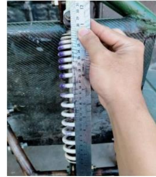
Figure 17. Spring Deflection Measurement
