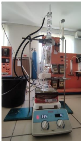
FIGURE 1. Coriander Seed Oil Extraction Process Soxhlet Extraction
